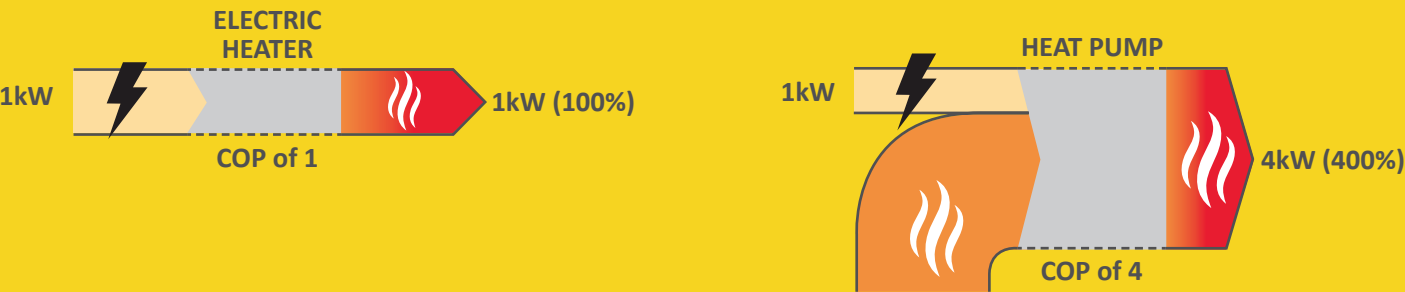
Figure 6 Coefficient of performance of an electric heater on the left, heat pump on the right. The 3kW of ambient heat from the ground heat exchangers (here in orange) makes the difference.
