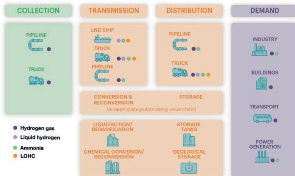
Figure 5: storage, transmission and distribution of hydrogen (Source: IEA (2019) [8: p68])
